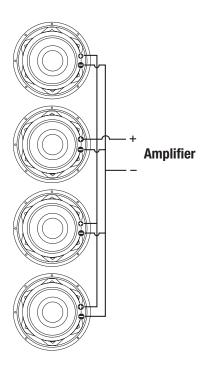
Parallel wiring of four single 4 ohm subs = 1 ohms
