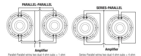
NOTE: Never connect only one coil of a Dual Voice Coil (DVC) speaker. BOTH voice coils must be connected to the amplifier
