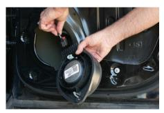
2. Remove the factory speaker by unclipping it at the top and pulling it forward. Then carefully unplug the speaker and remove the vehicle.
