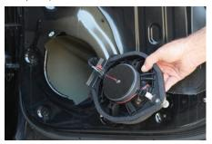
3. Plug in you new speaker and clip in starting from the bottom first. Securely mount the new speaker using the 7mm bolt. There are two extra mouting holes at the bottom of the speaker that will require drilling new holes to use. These are optional mounting holes
