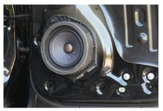
Remove door panel to gain access to the factory speaker. Remove the 7mm bolt at the top of the speaker (do not discard this bolt as you will need it to install your new speaker).
