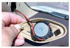
2. Unclip or remove factory tweeter from pillar or panel.
