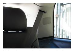
REAR 1. Remove panel to gain access to the factory speaker. Carefully unplug and remove panel and speaker.
