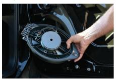
3. Plug in you new speaker and clip in starting from the bottom first. Securely mount the new speaker using the 7mm bolt. There are two extra mounting holes at the bottom of the speaker that will require drilling new holes to use. These are optional mounting holes.
