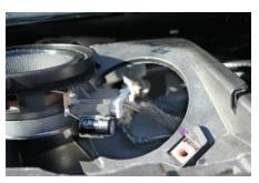
FRONT 2. Plug in and mount your new speaker with the screws you removed from the factory speaker.
