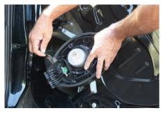
2. Remove the factory speaker by unclipping it at the top and pulling it forward. Then carefully unplug the speaker and remove from vehicle.
