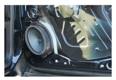
1. Remove door panel to gain access to the factory speaker. Remove the 7mm bolt at the top of the speaker (do not discard this bolt as you will need it to install your new speaker.
